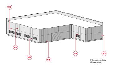
A vertical sandwich panel system that comes complete with accessories for jointing, windows, doors and gateways
