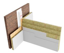
For closing the junction between a party wall and the external cavity, SCB is available in a larger 200mm width.
